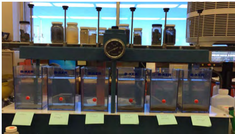
Clarified FGD wastewater following chemical precipitation with lime, ferric chloride, and organosulfide
